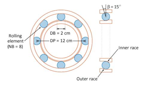
With the above physical dimensions of the bearing, visualize the fault frequency bands using bearingFaultBands.
