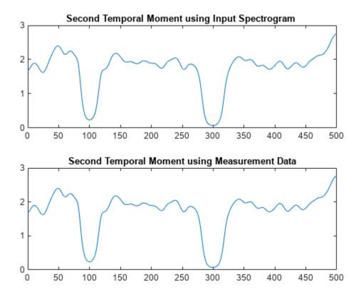
As expected, the plots match since the default pspectrum options were used for both. This result demonstrates the equivalence between the two approaches when there is no customization.
