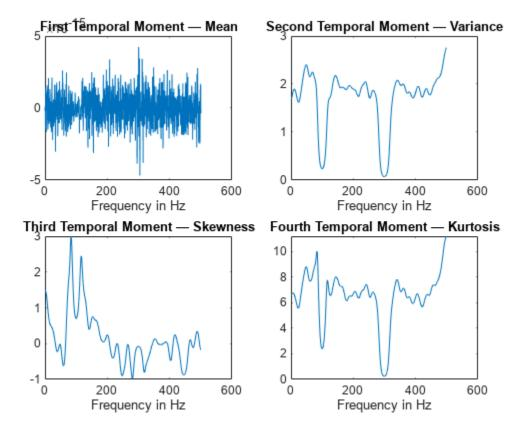
For the data in this example, the second and fourth temporal moments show the clearest features for the faulty resonance.
