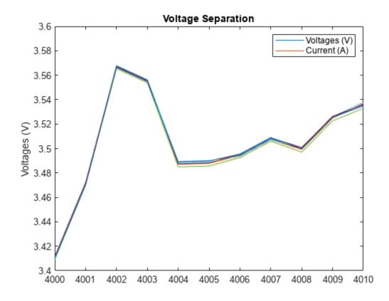
The voltages track closely together. There is no cell that is obviously degrading relative to the others. Identify the worst cell using meanDifferenceModel. meanDifferenceModel(internalShortCircuit(:,2:end))
