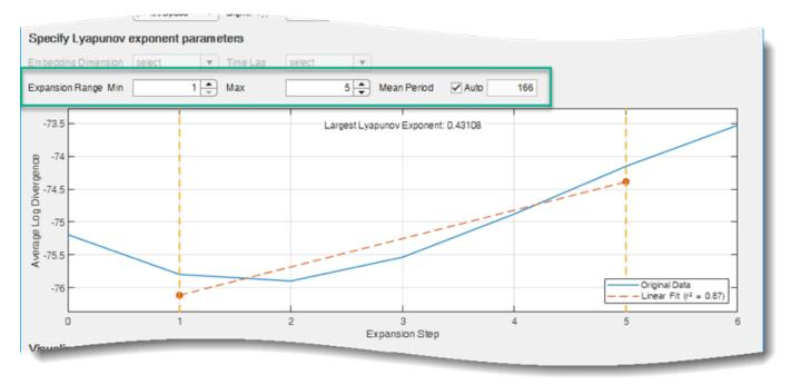
If your linear fit line does not align with the original data line using the default expansion range values, try different values in the **Expansion Range Min**, **Expansion Range Max** and **Mean Period** fields until the alignment is satisfactory. For this example, use the minimum value of 3 and maximum value of 7 for the best alignment. The default mean period value of 166 provides good alignment for the signal phaseSpace.
