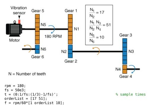
In practice, you would use measured data such as vibration signals obtained from an accelerometer. For this example, generate TSA signal X, which is the simulated data from the vibration sensor mounted on the motor.
