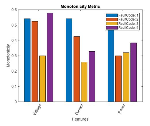
monotonicity returns a histogram plot with the features ranked by their monotonicity values. A higher monotonicity value indicates a more suitable prognostic parameter. For instance, the candidate feature Current has the highest monotonic trend for machines with FaultCode 1.
