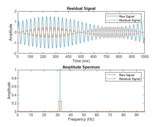
From the plot, observe the waveform and amplitude spectrum of the residual and raw signals, respectively.
