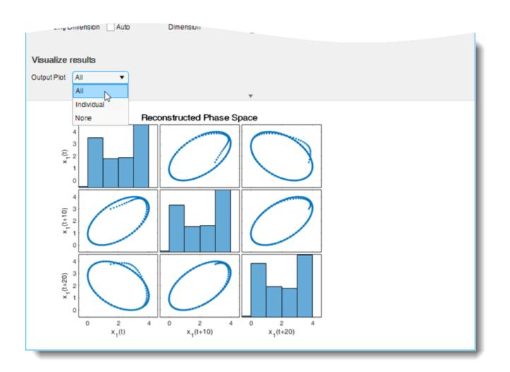
The task generates code in your live script. The generated code reflects the parameters and options you select, and includes code to generate the type of plot you specify. To see the generated code, click at the bottom of the task parameter area. The task expands to display the generated code.
