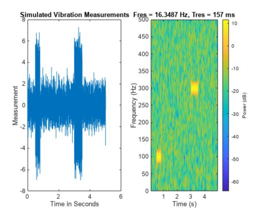
The spectrogram shows that the first burst is at 100 Hz, and the second burst is at 300 Hz. The 300-Hz burst is stronger than the 100-Hz burst by 70 dB.
