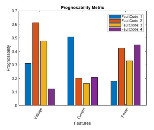
prognosability returns a histogram plot with the features ranked by their prognosability values. A higher prognosability value indicates a more suitable condition indicator. For instance, the candidate feature Current has the highest degree of prognosability for machines with FaultCode 1.
