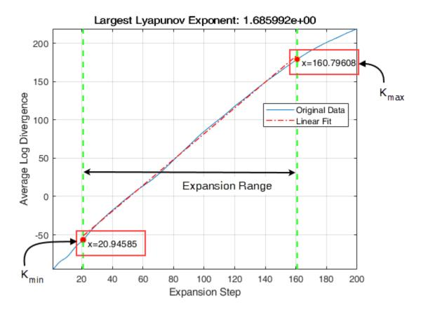
Note the new values of the expansion range after dragging the two vertical lines for an appropriate fit.
