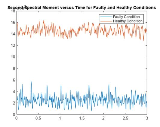
The moment plot shows behavior different from the earlier vibration plot. The vibration data for the faulty case is much noisier with higher-magnitude spikes than for the healthy case, although both appear to be zero mean. However, the spectral variance (second spectral moment) is significantly lower for the faulty case. The moment of the faulty case is still more noisy than the healthy case.
