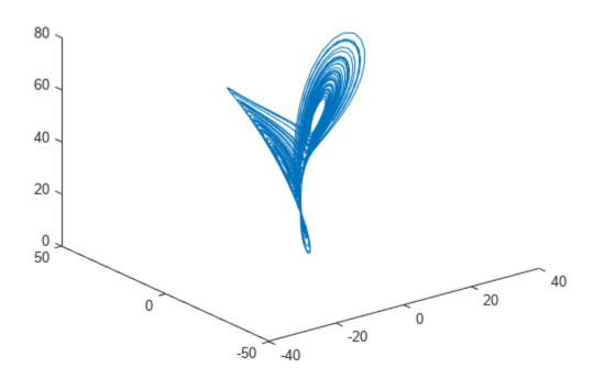
For this example, use the x-direction data of the Lorenz attractor. Since Lag is unknown, estimate the delay using phaseSpaceReconstruction. Set dimension to 3 since the Lorenz attractor is a threedimensional system. The dim and lag parameters are required to create the logarithmic divergence versus expansion step plot.
