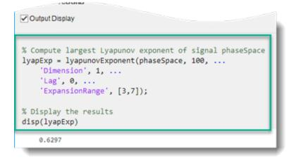
By default, the generated code uses lyapExp as the name of the output variable. To specify a different output variable name, enter a new name in the summary line at the top of the task. For instance, change the name to lExponent.
