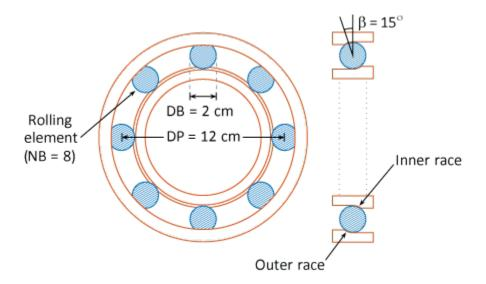
With the above physical dimensions of the bearing, construct the frequency bands using bearingFaultBands.
