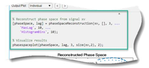
By default, the generated code uses phaseSpace as the name of the output variable. To specify a different output variable name, enter a new name in the summary line at the top of the task. For instance, change the name to pSpace.
