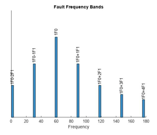
To avoid truncating negative fault frequency bands, set 'Folding' to true to fold them onto the positive frequency axis.
