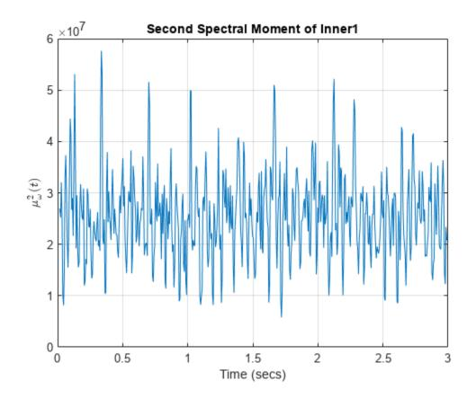
The plot illustrates the changes in the variance of the x\_inner1 spectrum over time. You are limited to this visualization (moment versus time) because tfsmoment returned no data. Now use tfmoment again to compute the second spectral moment, this time using the syntax that returns both the moment values and the associated time vector. You can use the sample rate directly in the syntax (sr\_inner1), rather than the time vector you constructed (t\_inner1).
