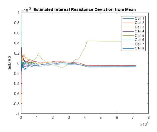
Cell 5, which the function identifies as the worst cell, has the largest internal resistance deviation.
