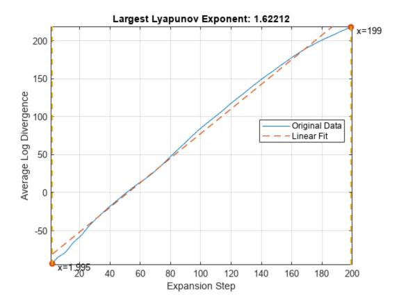
The first dashed, vertical green line (on the left) indicates the minimum number of steps used to estimate the expansion range, while the second vertical green line (on the right), represents the maximum number of steps used. Together, the first and second vertical lines represent the expansion range. The dashed red line indicates the linear fit line for the data, within the expansion range.
