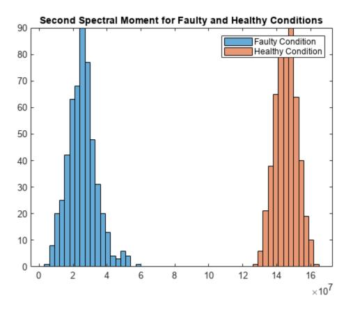
The moment behaviors distinguish the faulty condition from the healthy condition in both plots. The histogram provides distinct distribution characteristics — center point along x-axis, spread, and peak histogram bin.
