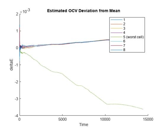
The mean difference model clearly differentiates cell 5.
