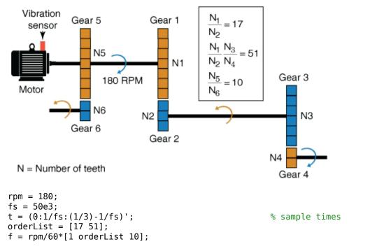
3 and 4 by specifying their gear ratios of 17 and 51 in orderList. The signal components corresponding to the shaft rotation (order = 1) is always implicitly included in the computation.
